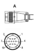
The front view of the 2 kW interconnection cable is shown above.
